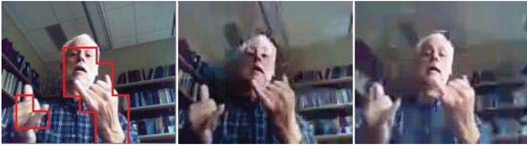
Fig. 5. A snap shot of ROI-based Encoder (a) original frame with skin blocks (red lines) (b) 0 ROI (c) 12 ROI. The quality in skin blocks is enhanced and quality in the rest of blocks is degraded.
