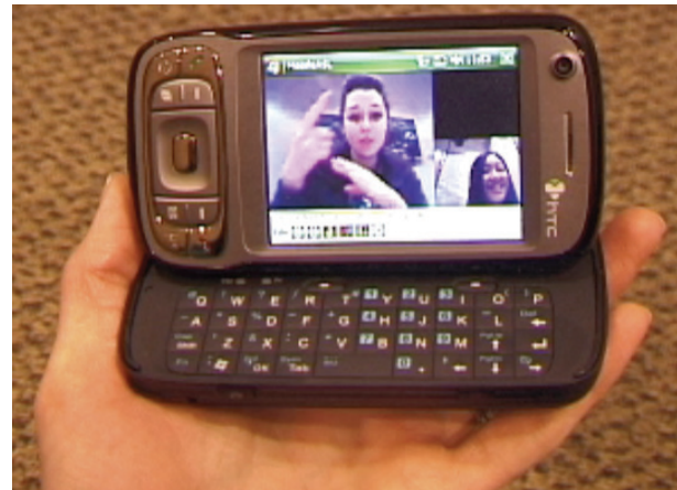
Figure 1: Deaf people can use MobileASL to communicate via real-time video on an off-the-shelf mobile phone over current non-3G cell phone networks.
